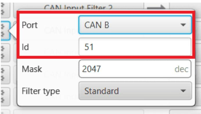
**CEX PDI Builder - CAN Input Filter configuration**
