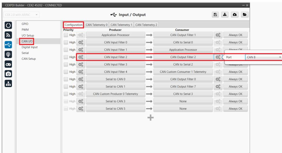
**CAN tunnel - CAN Output Filter configuration**
