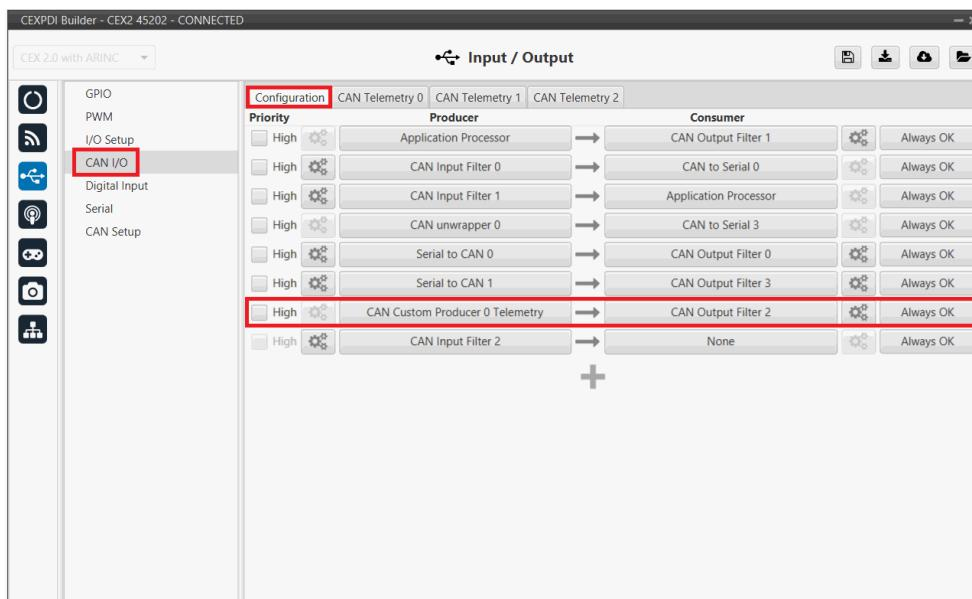
**CAN messages transmission - CAN I/O configuration**
